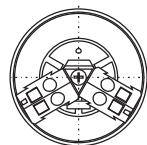
Single-phase capacitor with d = 60/70 mm Spring tension terminal AKD 25/2 for 2 × 6 mm 2 Art.-No. 31-08002
