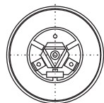
Single-phase capacitor with d = 60/70 mm For connection with flat cable plug 6.3 × 0.8 mm
